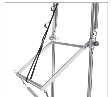
Figure 6: Safety strap holding the push-through bar at 4 o'clock. The strap is secured to the PTB and canopy frame, not the eyebolts.
