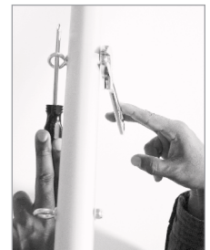
Figure 9: Use two fingers to tighten bolts
